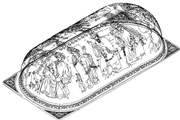
Il. 17. Saturio Estebarez, CONSULTING TOPOGRÁFICO S.L., drawing, 1999. Photogrammetric survey. 3D display of vault B2. Tracing of the important figures in the painting of this vault that gives it the name of the Hall of the Kings.
