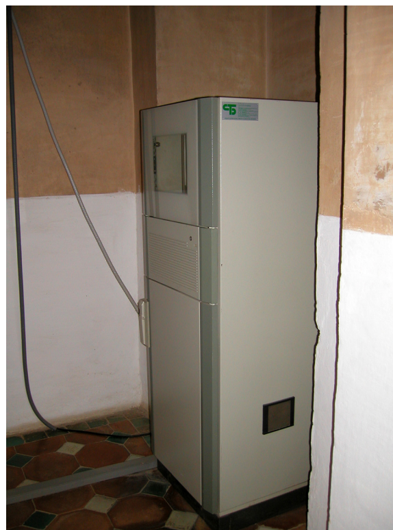
Il. 18. Pedro Salmerón Escobar, 2003, photography. Micro-climate point installed in the Hall of the Kings for initial environmental monitoring (agreement with the IAPH).
