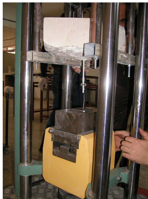
Il. 15. Pedro Salmerón Escobar, 2007, photography. Testing of the tensiometer and anchoring of the suspension system used in muqarnas domes M2, M4 and M6. Test carried out by Juan de Mata Vico Rodríguez in the laboratories of the Granada School of Architectural Technology laboratories (now ETS Building Engineering).
