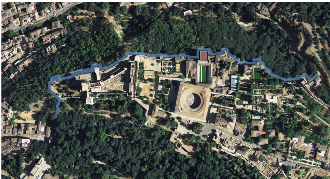
IL. 11. Safety perimeter against fire, 5 meters from the wall
