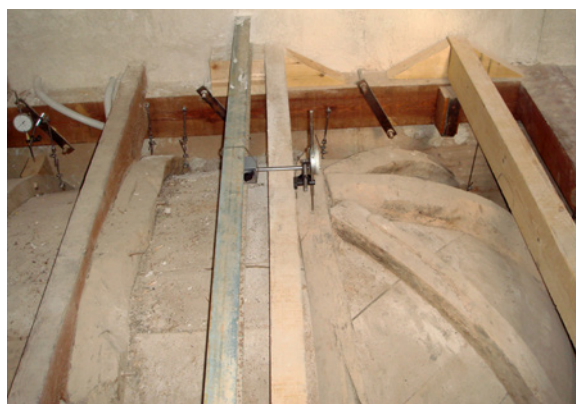
Il. 28. Pedro Salmerón Escobar, 2008, photography. View of the suspension system used in vault B1, reusing the wooden beams installed in the 1976–1983 restoration. Extensometers used in the load test can be seen.
