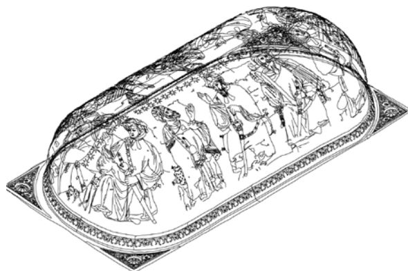
Il. 17. Saturio Estebanz, CONSULTING TOPOGRÁFICO S.L., drawing, 1999. Photogrammetric survey. 3D display of vault B2. Tracing of the important figures in the painting of this vault that gives it the of the Hall of the Kings.
