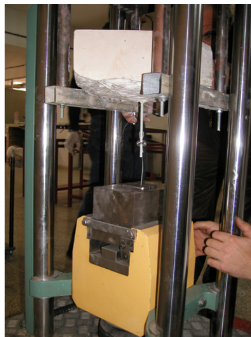
Il. 15. Pedro Salmerón Escobar, 2007, photography. Testing of the tensioner and anchoring of the suspension system used in muqarnas domes M2, M4 and M6. Test carried out by Juan de Mata Vico Rodríguez in the laboratories of the Granada School of Architectural Technology laboratories (now ETS Building Engineering).
